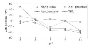
Fig. 2 – Zeta potential of NpAg\_silica, Ag^+\_phosphate, and Ag^+\_bentonite and (-x-) TiO\_2.
