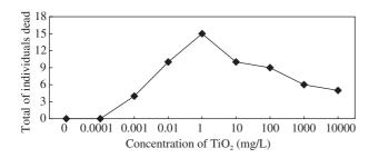
Fig. 3 – Total of dead D. magna after 48 hr in contact with  $TiO_2$  suspensions.
