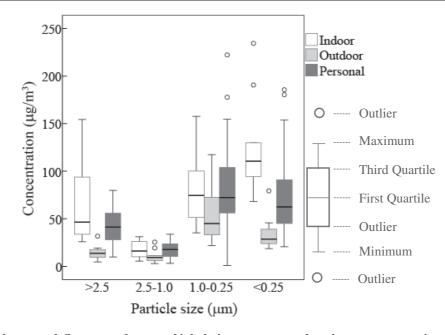
Fig. 2 – Comparison between daily averaged personal inhalation exposure and stationery concentration range of size-resolved particulate matter (open circles denote outliers), fractionated by aerodynamic diameters >2.5  $\mu$ m, 1.0–2.5  $\mu$ m, 0.25–1.0  $\mu$ m and <0.25  $\mu$ m.
