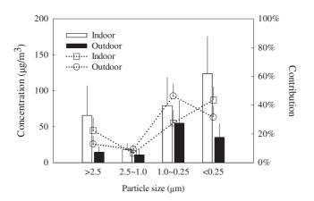
Fig. 1 – The 24-hr averaged mass concentrations of PM with different particle sizes (bar) and their contributions to TSP (line), fractionated by aerodynamic diameter at >2.5  $\mu$ m, 1.0–2.5  $\mu$ m, 0.25–1.0  $\mu$ m, and <0.25  $\mu$ m in indoor air and outdoor air.
