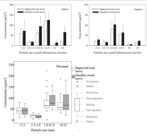
Fig. 4 – Comparison of size-resolved PM concentrations (µg/m<sup>3</sup>) between gasifier firewood stoves and improved coal stoves in Enshi County. Upper panel: stationary monitoring concentration; Lower panel: inhalation exposure concentration.
