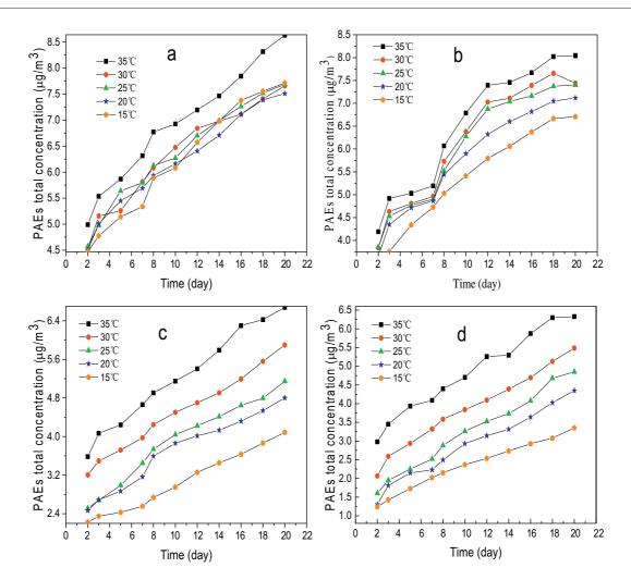
Fig. 3 – Emission concentration of total PAEs from plastic cups (a), plastic bags (b), plastic buckets (c) and Polyvinyl chloride (PVC) bag (d).
