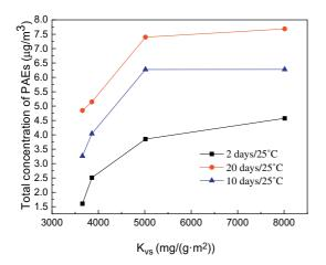
Fig. 5 – Concentration of total PAEs from different pollutant sources with different volatility strength coefficients at ambient temperature (25°C).
