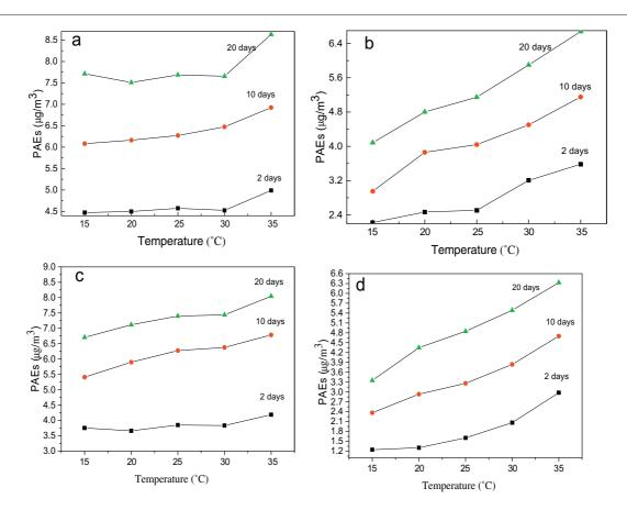
Fig. 4 – Emission concentrations of total PAEs from the plastic cups (a), plastic buckets (b), plastic bag (c), Polyvinyl chloride (PVC) bag (d) and in different closed times.
