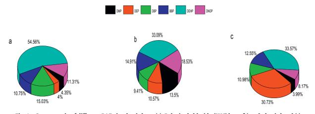
Fig. 1 - Content ratio of different PAEs in plastic bags (a), Polyvinyl chloride (PVC) bags (b) and plastic bowl (c).
