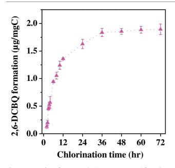
Fig. 4 – Formation of 2,6-DCBQ ( $\mu$ g/mg C ± SD; n = 3) from the chlorination of extracted total protein from C. *vulgaris*. Chlorination conditions: initial concentration = 30 mg/L as TOC, chlorine: TOC = 10:1, temperature = 25 ± 1°C. The concentration of 2,6-DCBQ was calculated on the basis of 30 mg/L TOC.
