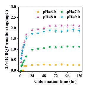
Fig. 1 – Formation of 2,6-dichloro-1,4-benzoquinone (2,6-DCBQ) ( $\mu$ g/mg C ± SD; n = 3) from chlorination of C. *vulgaris* determined using an HPLC-UV method. Chlorination conditions: initial algal cell concentration = 30 mg/L as total organic carbon (TOC), chlorine:TOC = 10:1, temperature = 25 ± 1°C. The concentration of 2,6-DCBQ was calculated on the basis of 30 mg/L algal TOC.
