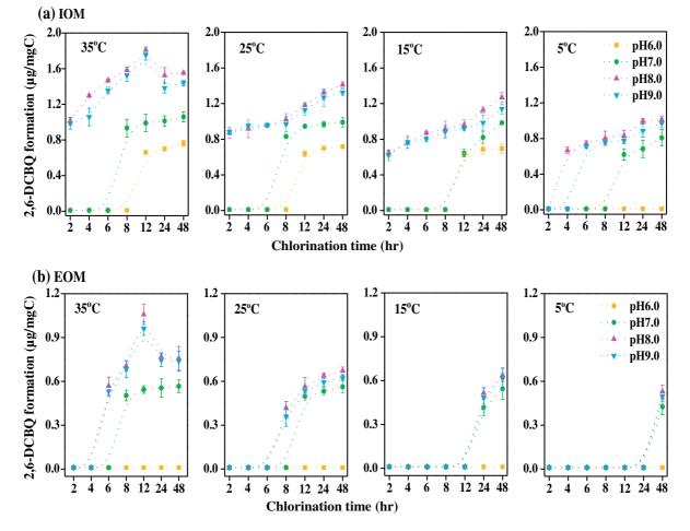
Fig. 2 – 2,6-DCBQ formation ( $\mu$ g/mg C ± SD; n = 3) from the chlorination of (a) intracellular organic matter (IOM) and (b) extracellular organic matter (EOM) fractions of *C. vulgaris* under variable pH and temperature conditions.
