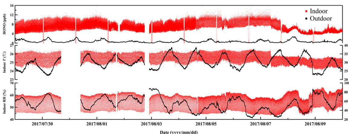
Fig. 2 – Time series of indoor and outdoor HONO, relative humidity (RH), and temperature (T) in the laboratory of ICCAS during the observation period from July 29 to August 9, 2017.
