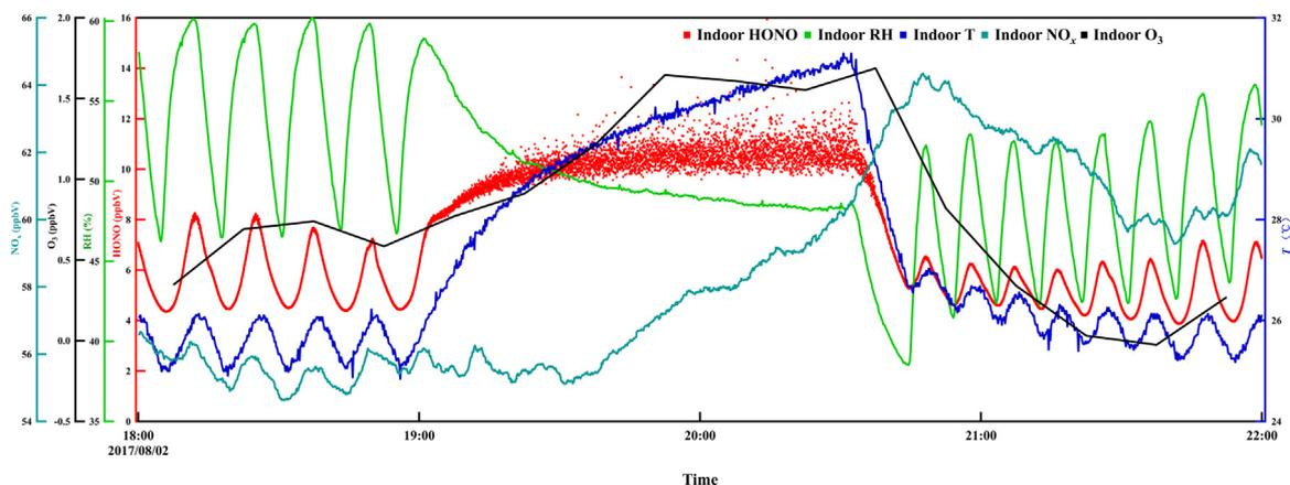
**Fig. 3 – Temporal variations of indoor HONO, NO<sub>x</sub>, O<sub>3</sub>, RH, and T during the period when the air conditioner was turned off in the laboratory of ICCAS.**
