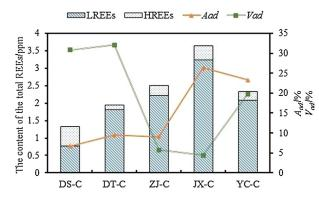
Fig. 3 – The relationship between the contents of REEs in the coal-burning  $PM_{10}$  (C) and ash yields, volatile contents in the raw coals. Note:  $A_{ad}$  is ash yields,  $V_{ad}$  is volatile contents, ad represents air dry base.
