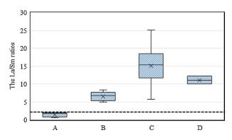
Fig. 4 – Box-plot showing comparison of the La/Sm ratios in particulate matter from different sources. Note: A represents the emission of laboratory coal-burning system in this study, B represents the ambient indoor coal-burning environment (Hu, 2016), C represents the tunnel environment dominated by gasoline vehicle emission (Hou, 2017), D represents the gasoline-powered vehicles emissions by engine test bench (Xing, 2018).
