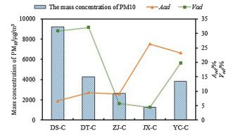
Fig. 2 – The relationship between the mass concentration of the coal-burning  $PM_{10}$  and moisture contents, ash yields, volatile contents in the raw coals. Note: " $M_{ad}$ " is moisture content, " $A_{ad}$ " is ash yield, " $V_{ad}$ " is volatile content, "ad" represents air dry base.
