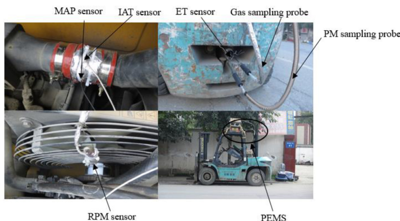
Fig. 2 – Installation of the PEMS used in this study to a forklift for emissions measurements.
