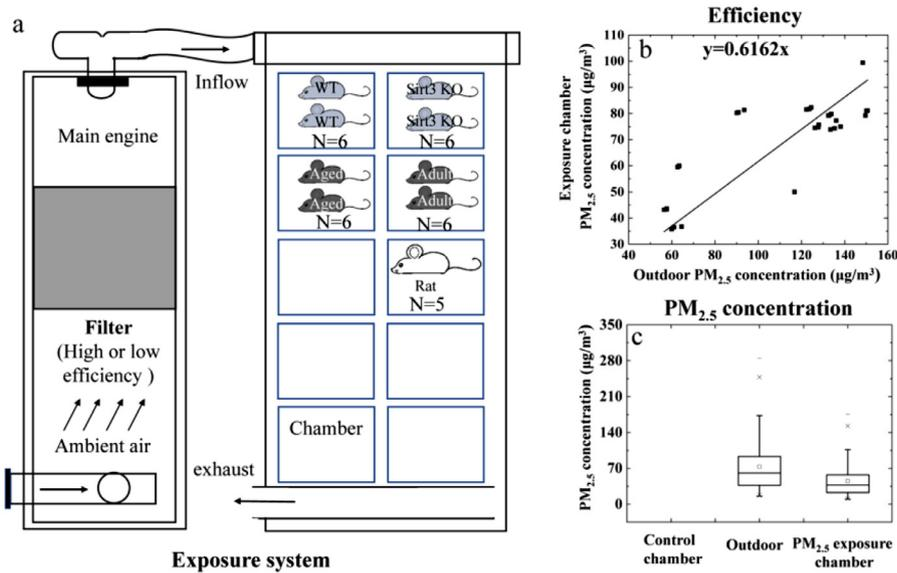
**Fig. 1.** – Real-ambient PM<sub>2.5</sub> exposure system. (a) Schematic diagram of the exposure system; (b) linear regression of PM<sub>2.5</sub> concentrations in and out of the exposure chambers; (c) average PM<sub>2.5</sub> concentration in the control and exposure chambers during the exposure period (21/01/2019–05/05/2019).
