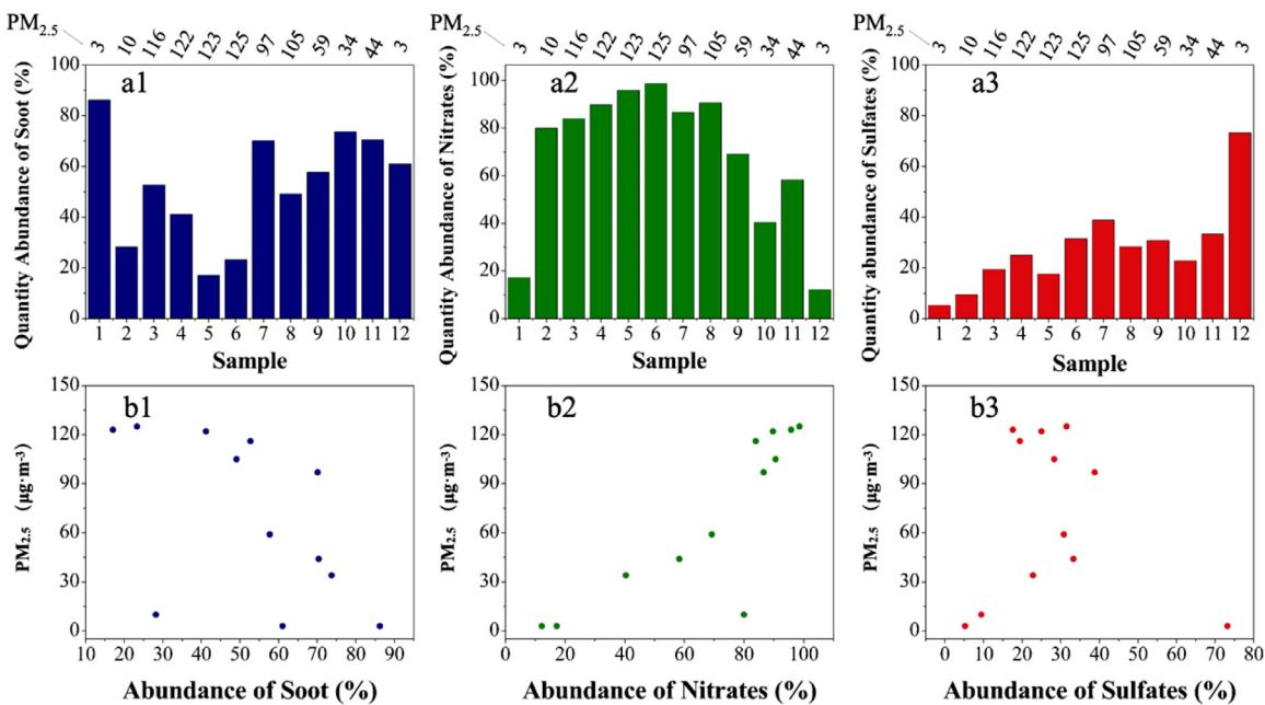
**Fig. 3 – (a1-a3)** Relative abundance of soot, nitrates, and sulfates during the haze event. **(b1-b3)** Relationship between PM<sub>2.5</sub> mass concentration and the abundance of soot, nitrates, and sulfates.
