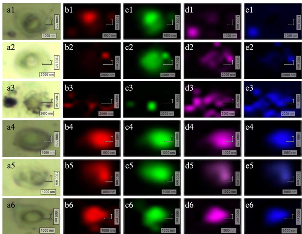
**Fig. 5 – Mapping analysis of the mixing state of fine particles on clear days (a1–e3) and hazy days (a4–e6). (a)** Raman optical image of fine particles and the Raman mapping signals of: **(b)** sulfates (red), **(c)** nitrates (green), **(d)** the D-band (magenta), and **(e)** the G-band (blue).
