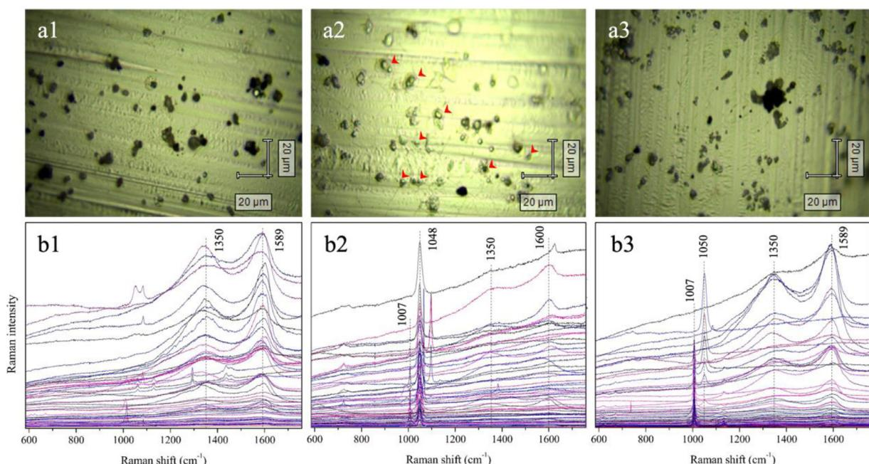
**Fig. 2 – Surface-enhanced Raman scattering (SERS) spectrum corresponding to samples collected before, during, and after the haze event (1–3, respectively). (a1–a3) Raman optical images of PM<sub>2.5</sub> particles (red arrows in a2 indicate core-shell structures), and (b1–b3) SERS spectra of individual PM<sub>2.5</sub> particles.**
