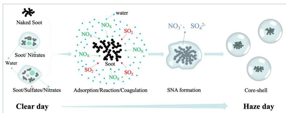
**Fig. 6 – Conceptual graph showing the mechanism for the production of the core-shell structure of PM<sub>2.5</sub>.**
