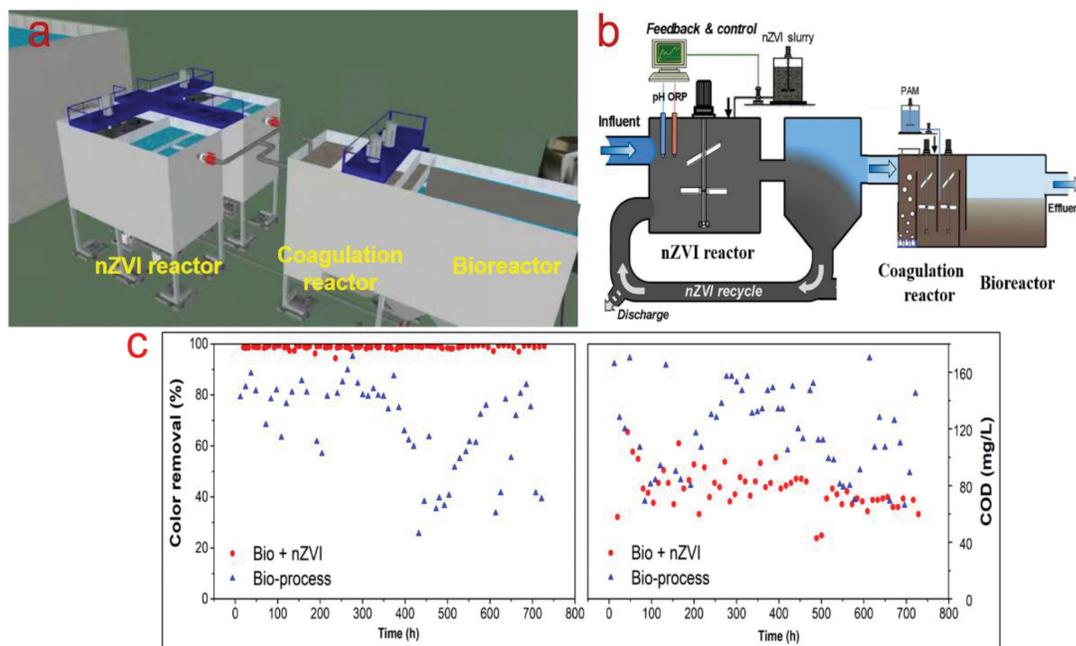
**Fig. 2 – An example of the combined nZVI and biological process to treat industrial wastewater: a) the combined treatment plant showed in 3-D schematic. b) schematic process illustrated in 2-D process. c) efficiency of color removal and COD reduction.**
